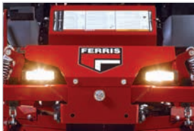
Light Kits Pre-wired kit and new kits with a wire harness for simple installation. (Select models)
