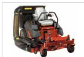
Turbo-Pro™ Collection System 227 Liter hard-top collection system with air-assist turbo.
