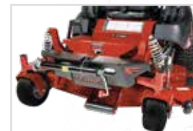
Front Bumper Kit With integrated 2x 6 Watt LED lights, weight- and service jack mount. (Service jack sold separate)
