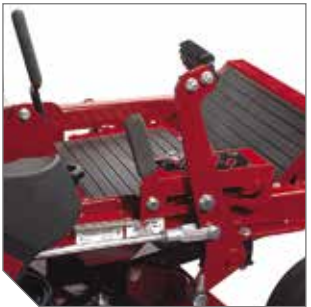
Foot-operated deck lift, with adjustable pedal, can change cut height in 1/4" increments from 1.5" - 4.5".
