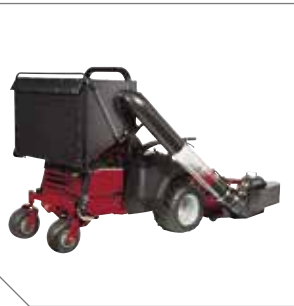
Shown with optional FAST-Vac™ EZ Dump XL™ Grass Collection System. Capacity: 14 cubic feet
