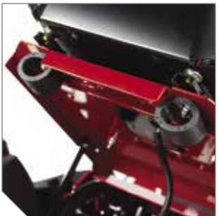
Isolation bumpers under the seat mount provides additional operator comfort.
