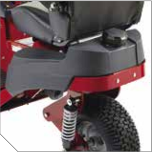
Rugged 5.5-gallon fuel tank with wide filler neck and reserve.
