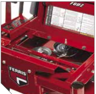
Quick removal of the floor pan provides convenient access to the top of the deck for easy cleaning and service.
