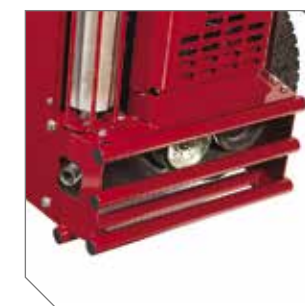
Heavy-duty integrated rear bumper protects engine compartment.
