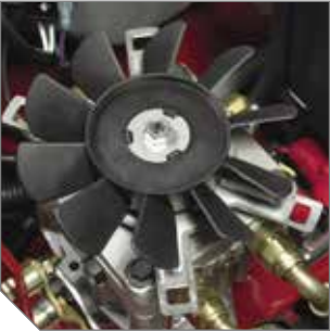
Fan mounted on top of hydro pump assists in cooling of hydro system and repelling debris.
