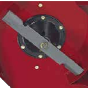
Marbain® Steel Blades Our exceptionally strong 1/4" thick blades generate greater lift for a precision cut and require less frequent sharpening.
