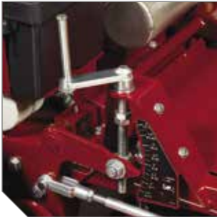
Quick-adjust height of cut control sets cut height in one easy step.
