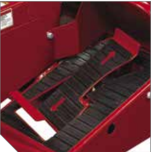
Foot pedal controls speed and forward / reverse direction.
