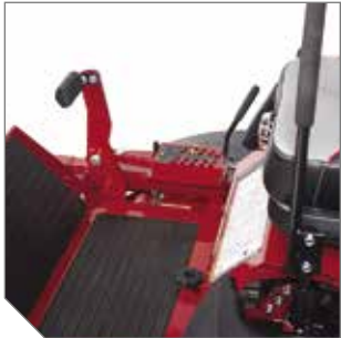
Foot-operated deck lift, with adjustable pedal, can change cut height in 1/4" increments from 1.5" - 6".
