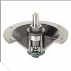
Hercules™ II Spindles Industrial 10" dia. cast-iron spindle assembly with 1 3/16" dia. shaft and greaseable double row angular contact ball bearings, which can be greased through the convenient top access grease fitting.
