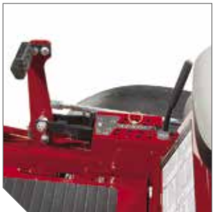
Foot-operated deck lift, with adjustable pedal, can change cut height in 1/4" increments from 1.75"- 5".
