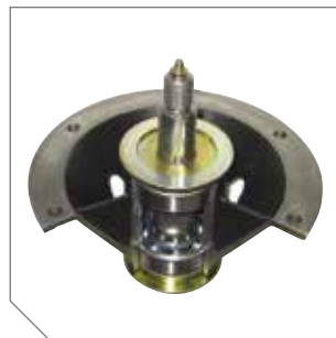
Cast-Iron Spindles longer usable life, 1" shaft with top access grease fitting for greaseable dual ball bearings, six-bolt 8" flange design adds strength and greater dispersal of energy to deck assembly.
