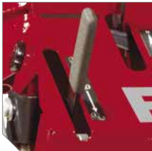
Brake handle is conveniently located beside the control panel, providing instant access with minimal operator effort to engage.
