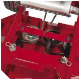
Deck drive belt system and larger pulleys provide gentler belt tension, which – combined with our unique debris shield – extends belt life and reduces wear on bearings.
