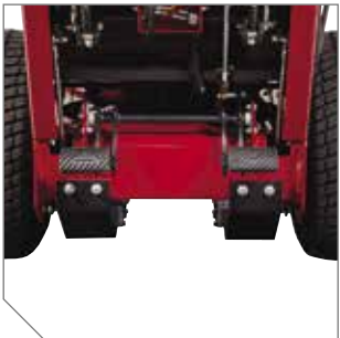
Centralized foot control for neutral position provides the operator with a more natural control.
