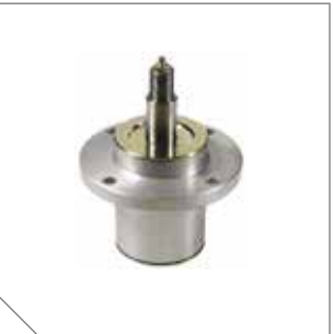
Aluminum Spindles feature 1" shaft with greaseable 2.5" x 1" dual ball bearings with top access grease fittings and pressure relief valve.
