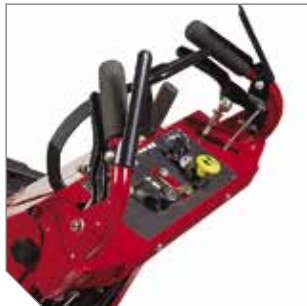
PTO switch allows operator to stop the blades simply by putting the mower in neutral position and releasing operator presence handles, while the engine continues to run.
