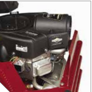
Heavy-duty bumper protects the engine while also allowing for easy service access.
