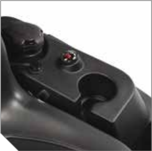
Ergonomic control panel features cup holder and fuel gauge for operator convenience.
