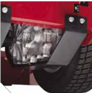
Heavy-duty transmission guards reduce build up of debris to improve air flow and allow for access to the filter for maintenance.
