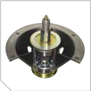
Cast-Iron Spindles longer usable life, 1" shaft with top access grease fitting for greaseable dual ball bearings, six-bolt 8" flange design adds strength and greater dispersal of energy to deck assembly. (52" Model)
