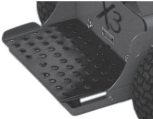
Step onto the operator platform, disengage parking brake, grasp the handle bar to operate the machine. Engage parking brake before stepping off the machine.
