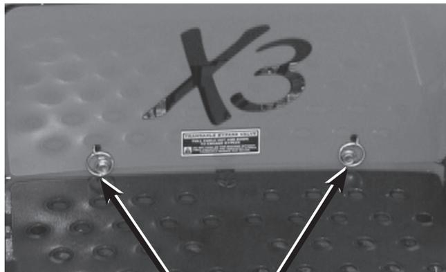
Hydraulic Pump Bypass Valves
