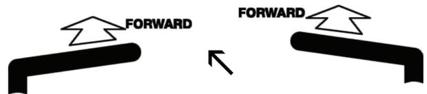
For a gentle left turn, Push the right motion control lever further forward than the left motion control lever.
