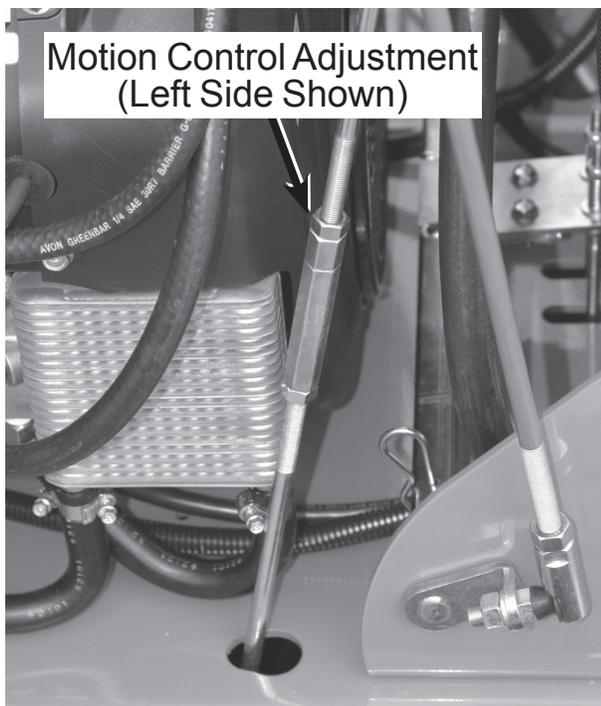
5. There are adjusters located by the transaxles on the control linkages. Loosen the jam nuts on the top and bottom of the adjuster.
