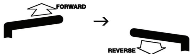
For a sharp right turn, Push the left motion control lever forward and pull the right motion control lever rearward.
