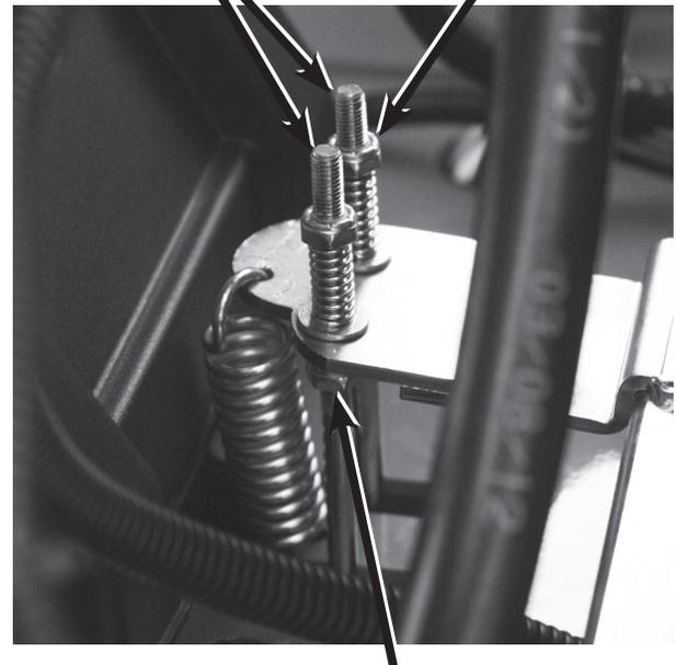
**Brake Release Adjusting Nut**
