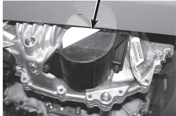
**Transaxle Drain Plug and Hydraulic Oil Filter.**
