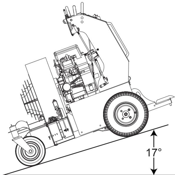
1. Stop machine on a 17° slope (30% grade) facing downhill. Stop the engine and engage parking brake.
