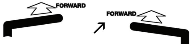
For a gentle right turn, Push the left motion control lever further forward than the right motion control lever.
