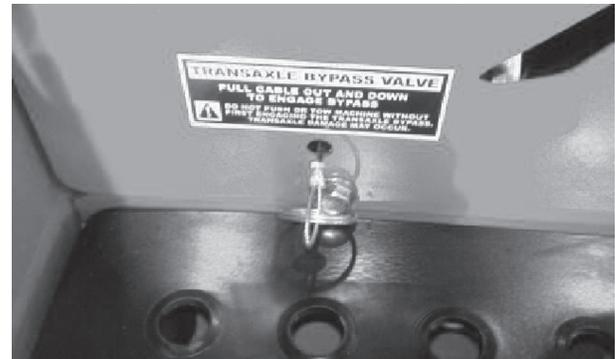
**Transaxle Bypass Valve Engaged**
