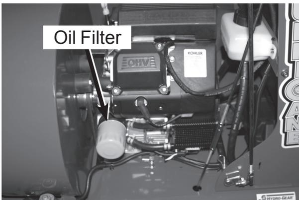
**IMPORTANT:** Make sure engine and exhaust system is cool before proceeding. The oil filter is located behind the muffler which can cause severe burns if the engine is hot.
