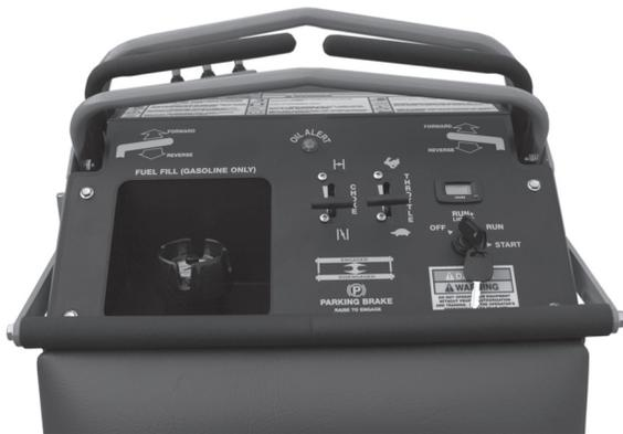
This photo shows the hydrostatic control levers are in the NEUTRAL position.
