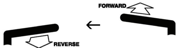
For a sharp left turn, Pull the left motion control lever rearward and push the right motion control lever forward.
