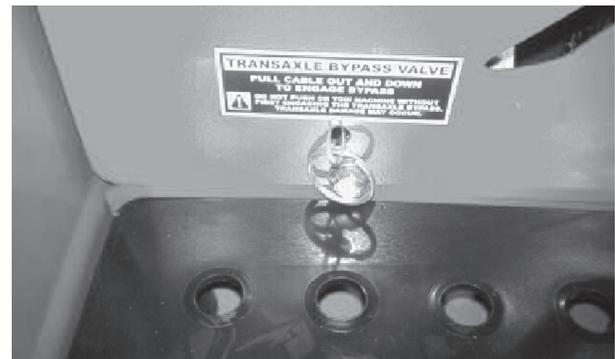
**Transaxle Bypass Valve Disengaged**
