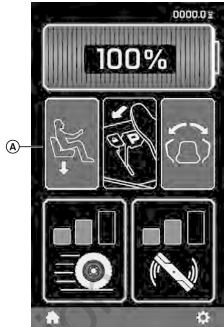
Drive Screen - System Fault Alert (Figure 13)
